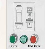
Pneumatic Controlled Cutter Holder Lock / Unlock
