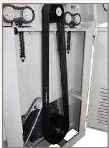
Powerful Cutterhead Drive Motor
