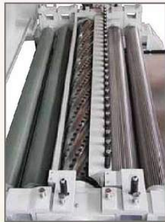
Rubber-covered Outfeed Rollers (Left) & Sectional Infeed Rollers (Right)
