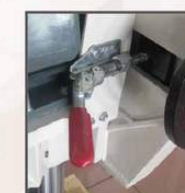
Built-in Manual Brake for quick stop
