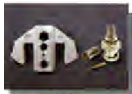
E1 DIE RG TYPE COAXIAL CABLE CONNECTOR 255/187/068/213" 6.48/4.75/1.72/5.41 mm RG 58, 59, 62, 174
