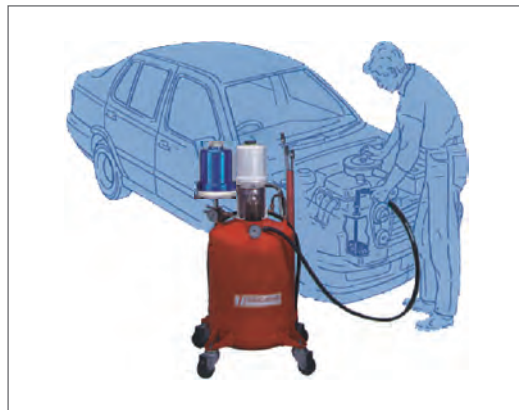
▲ Diagram of oil suction
