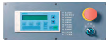
▲ S1 (SIEMENS PLC CONTROL)
