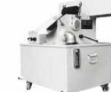
11. Magnetic separator w/ coolant system
