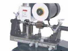
Sharpening gear hob held on C2T12 fixture with a AB01-AB04 arbor, C2R2 plain tooth rest is indexed against index disc
