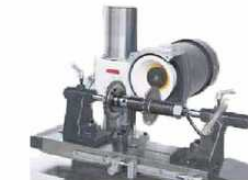
Sharpening side milling cutter held on C2T12 fixture with a AB01-AB04 arbor, C2R2 plain tooth rest is indexed against index disc
