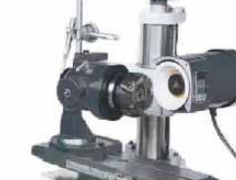
Sharpening face milling cutter being held in the C2SF fixture with a AA20-AA26 arbor, cutter is indexed with C2R1 univ tooth rest, and wheel is diamond cup wheel
