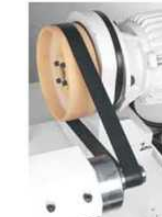
Automatic Belt Tension Control
