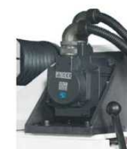
Spindle Head Driven by Servo Motor
