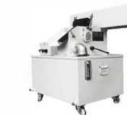
9. Magnetic separator w/ coolant system
