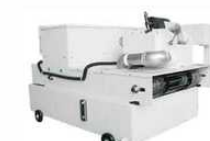
4. Auto paper strip filter & magnetic separator w/ coolant system
