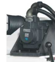
Spindle Head Driven by Servo Motor
