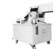
9. Magnetic separator w/ coolant system
