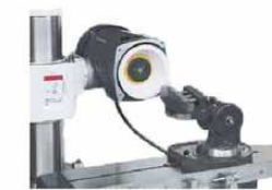
Sharpening turning tool set-up on C2LH fixture
