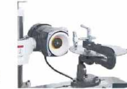
Sharpening circular saw blade held on C1SG attachment
